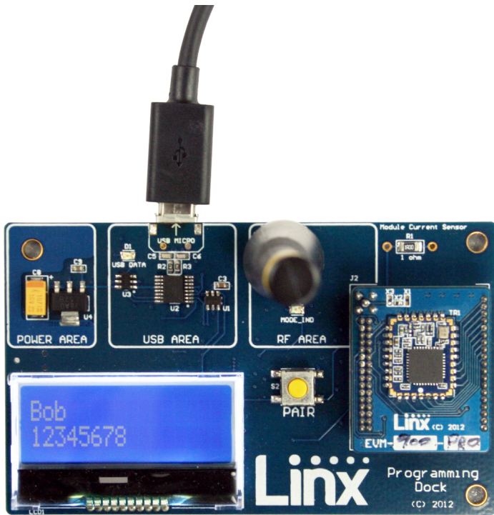
Figure 13: The Master Development System Programming Dock with Name and Address Displayed
